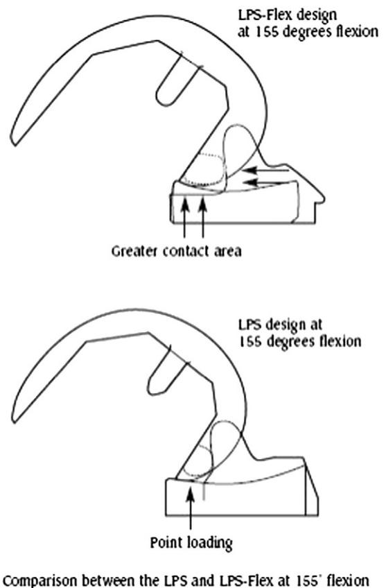
**Fig. 1.** The double arrows indicate the increased contact area in the flex design at 155°.
